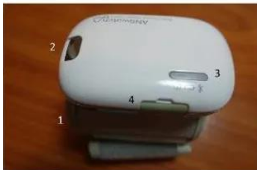
Figure 2. Name and function of ANS Watch (1) Wristband (contains biosensor) (2) Power switch (Power On-Off) (3) LED indicator (power on, test, charging, Bluetooth) (4) Micro-USB charging slot
